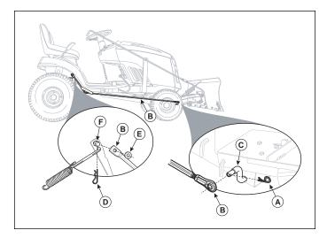
Figure 17. Control Arm Removal
